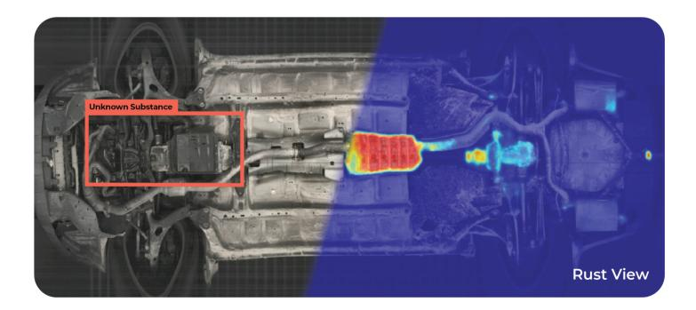
Wider view of the vehicle's undercarriage with the ability to view the frame & inner wheel.
